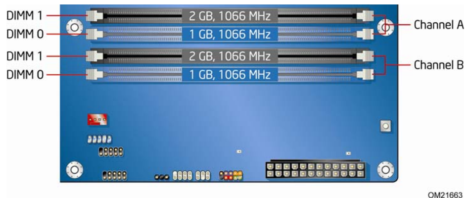
Figure 19. Example Dual Channel Memory Configuration with Four DIMMs
