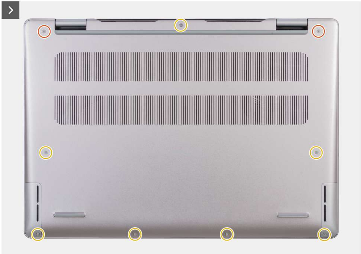
Figure 9. Removing the base cover
