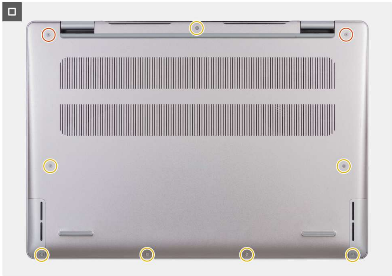
Figure 12. Installing the base cover
