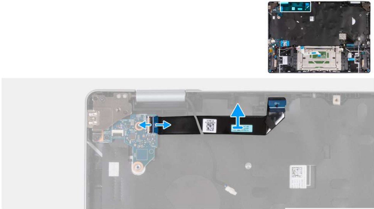
Figure 46. Removing the I/O-board cable
