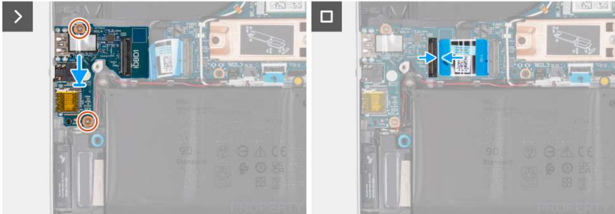
Figure 37. Installing the audio board
