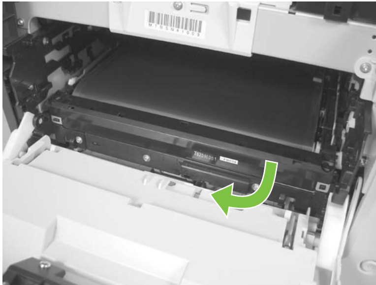
Figure 6-30 Remove the ITB (2 of 6)
