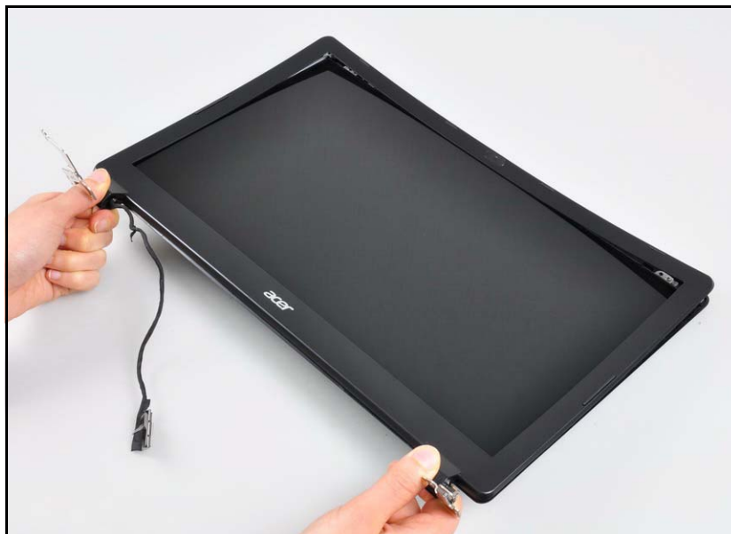
Figure 3-77. Replacing the LCD Bezel
