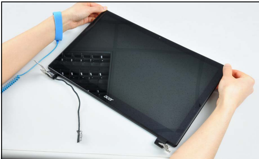
Figure 3-66. Replacing the Touchscreen LCD
