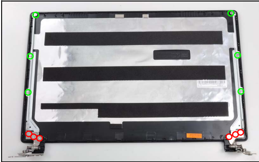
Figure 3-58. LCD Bracket Screw Location (Touchscreen)
