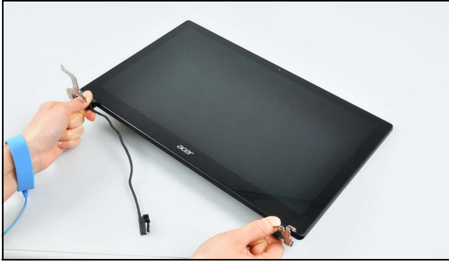
Figure 3-67. Replacing the Touchscreen LCD
