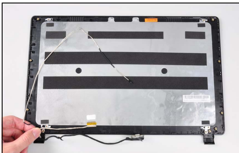
Figure 3-43. LVDS and Camera Cable Removal
