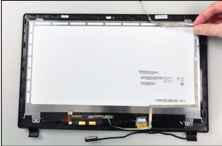
Figure 3-59. Replacing LVDS cable (Touchscreen)
