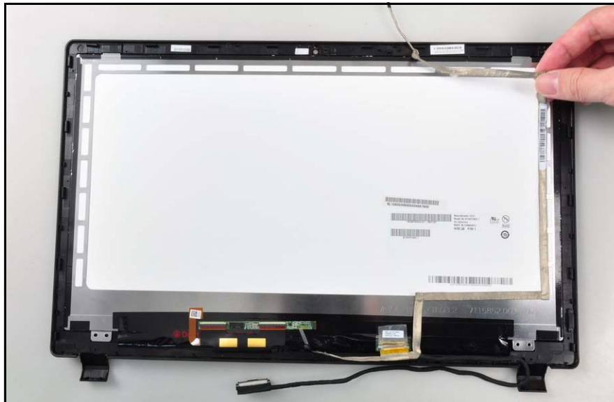
Figure 3-52. Removing LVDS cable (Touchscreen)
