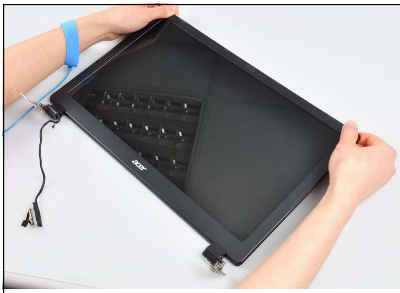
Figure 3-78. Replacing the LCD Bezel
