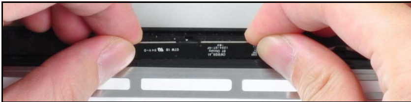
Figure 3-47. Lifting the Camera Module (Touchscreen)
