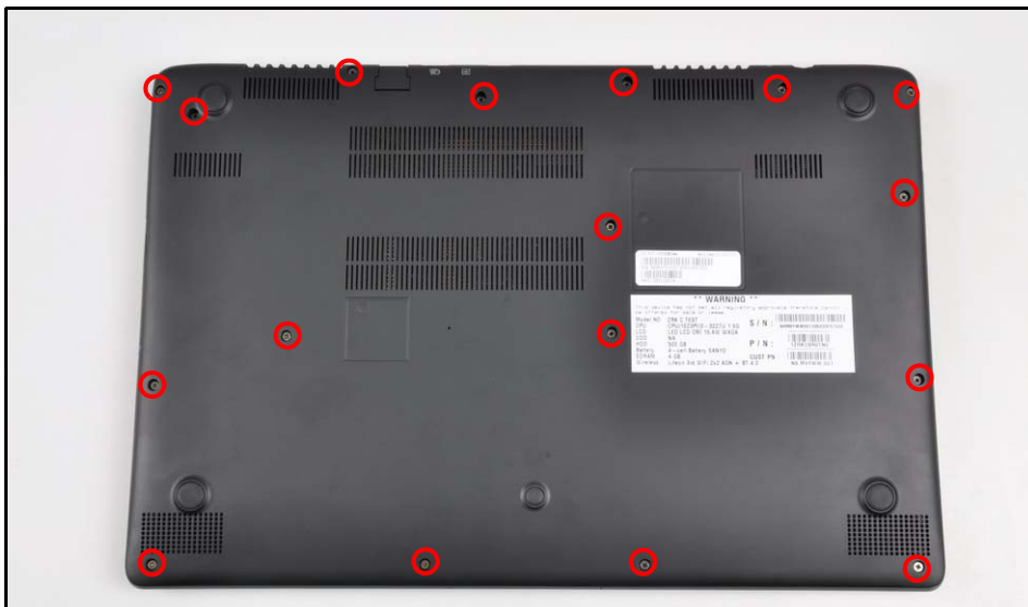
Figure 3-105. Base Cover Screw Location
