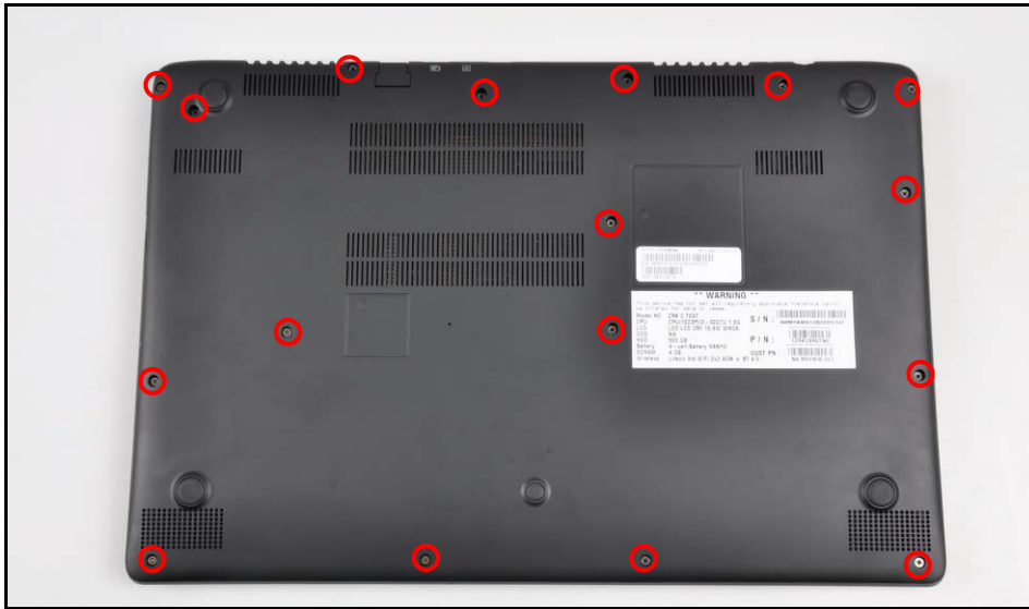
Figure 3-3. Base Cover Screw Location
