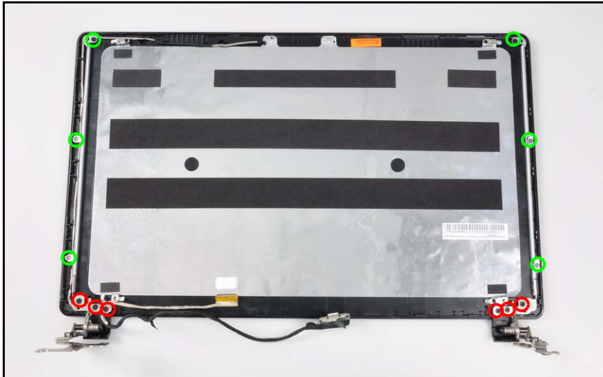
Figure 3-39. LCD Bracket Screw Location
