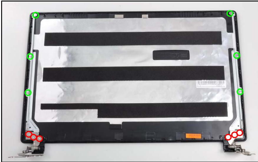
Figure 3-53. LCD Bracket Screw Location (Touchscreen)
