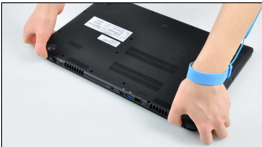
Figure 3-4. Base Cover Removal
