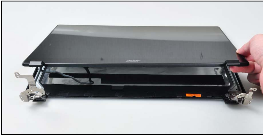
Figure 3-65. Placing the Touchscreen LCD
